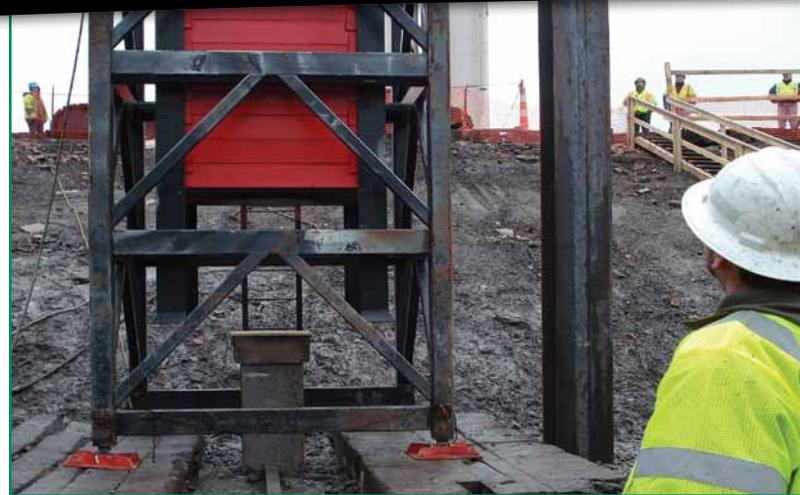
Dynamic Load Test with APPLE (red ram) on a steel H pile.
