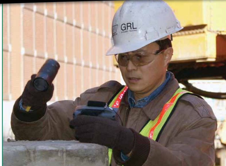
GRL engineer performing low strain dynamic testing.
