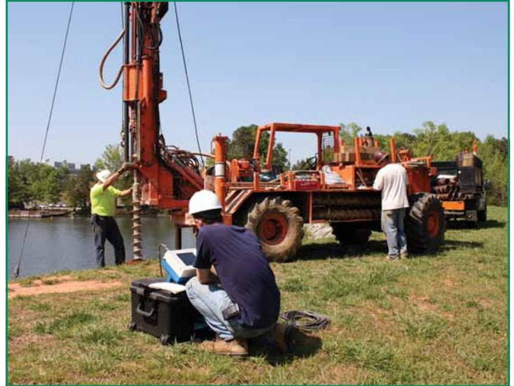
*GRL engineer calibrates an SPT hammer at Lake Raleigh.*
