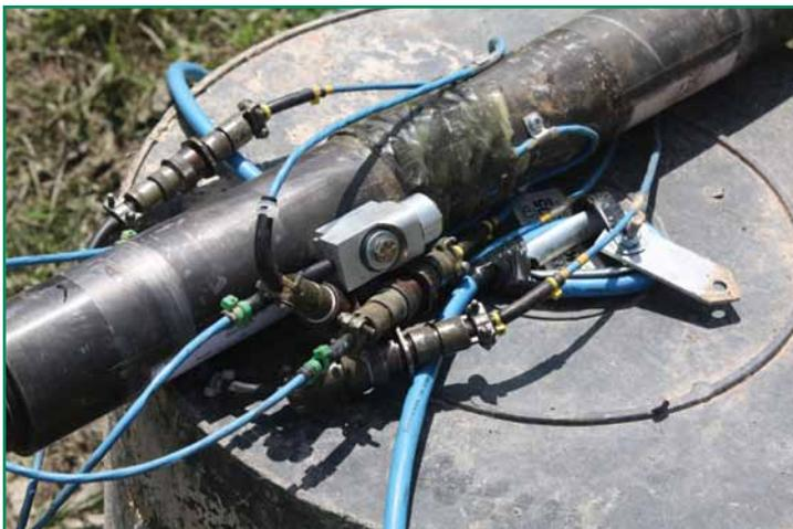
*SPT rod section instrumented with strain gages and accelerometers.*
