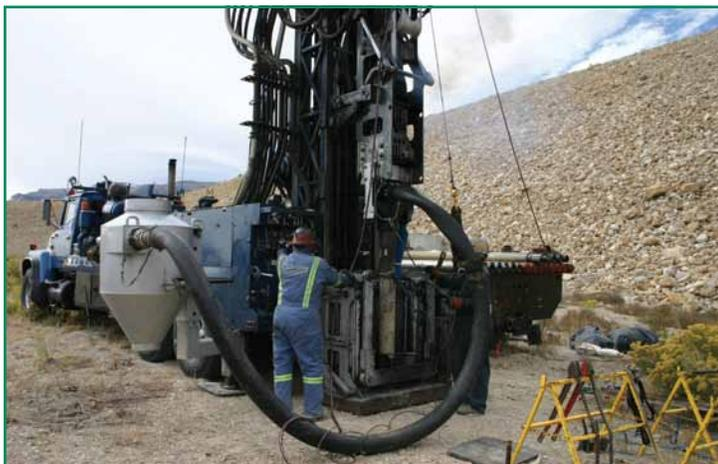
*Becker Test at Millsite Dam. These tests are common in liquefaction studies of dams and levees.*
