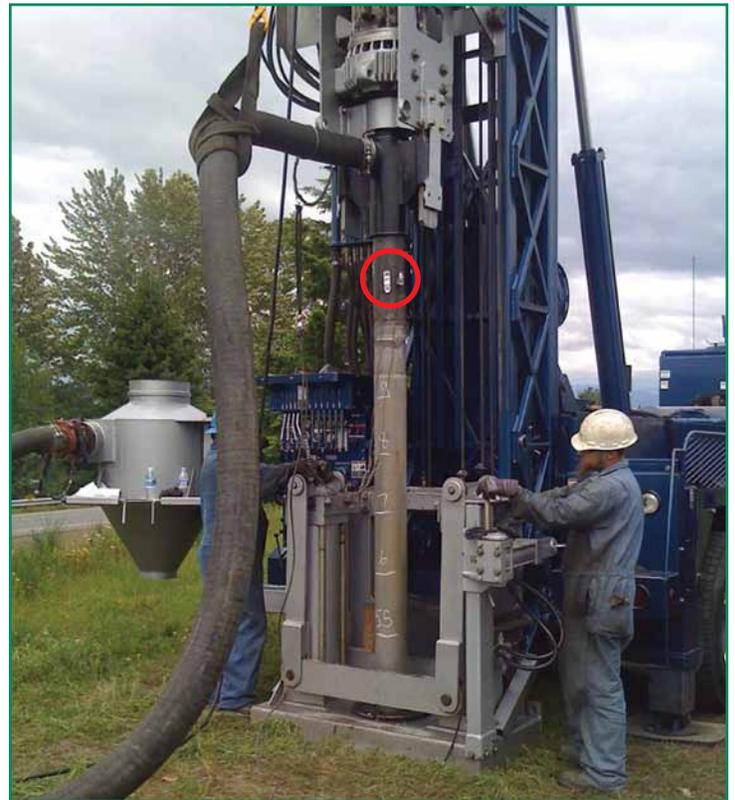
*Notice accelerometer and strain transducer near the top of the Becker casing.*
