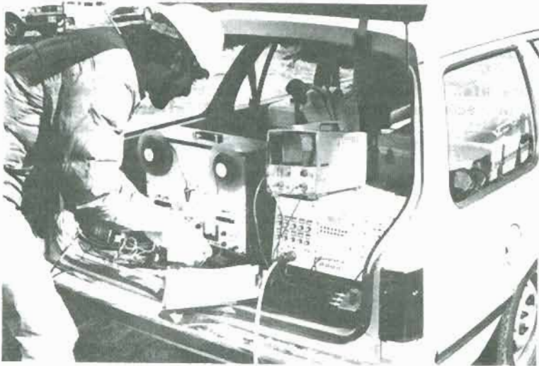
Figure 4: Photograph of the car-mounted field measurement equipment
