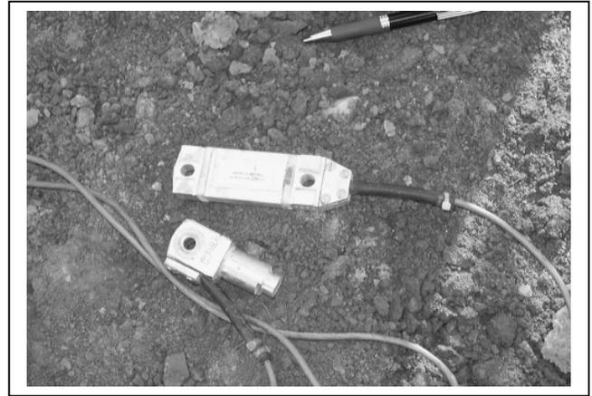
Fig. 4. View of the accelerometer and strain gauge used for PDA testing.
