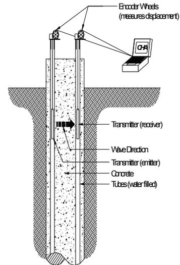
Fig. 4. Typical crosshole setup
