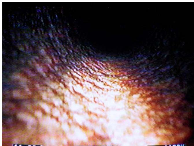
Fig. 8. Picture of intact concrete with microcamera
