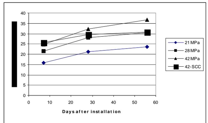
Fig. 8. PDI research shaft: concrete strength development.
