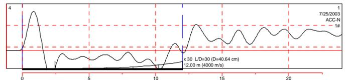
*Fig. 1: PEM record from a tower foundation*
