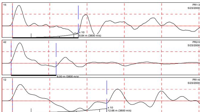
Fig. 2. PEM records from concrete piles under an existing bridge
