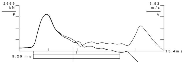
Fig. 4. PDA records of force and velocity from an H-pile with a cracked welded splice
