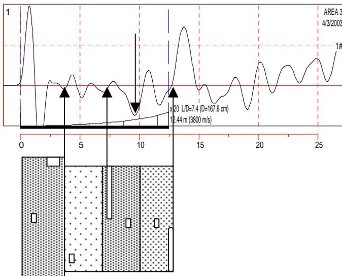
Fig. 5. PEM record and sketch of shaft with planned defects
