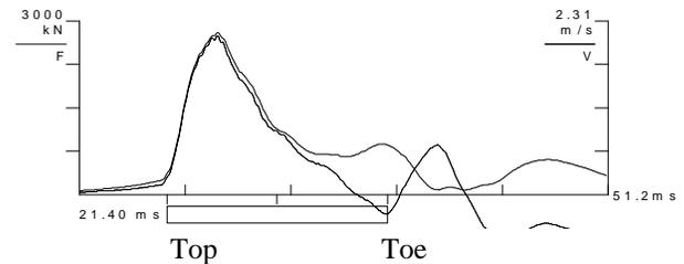
Fig. 3(a). Early PDA record of pile top force and velocity
