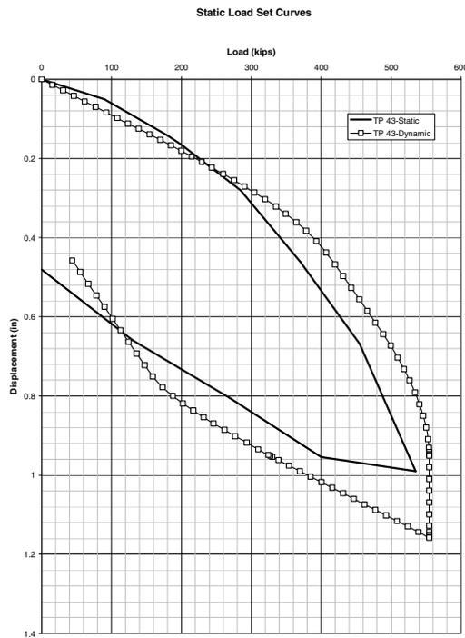
**Table 1.** Comparison of calculated with static test loads
