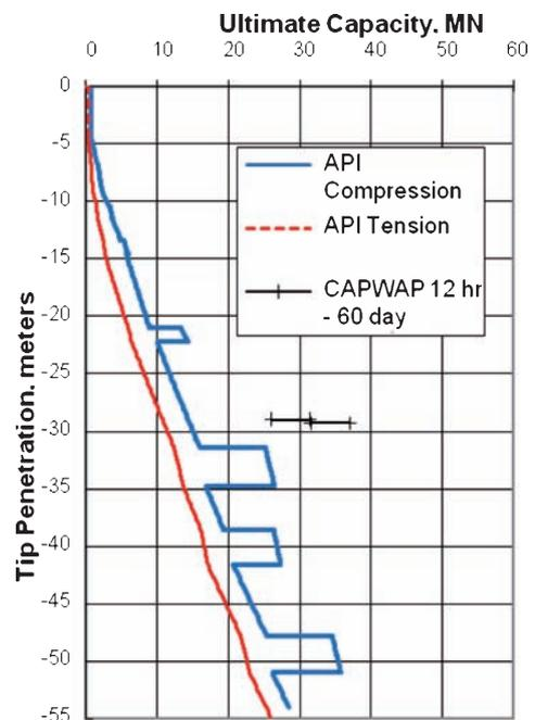
Figure 6. Site D Pile capacity from API and DMS results.
