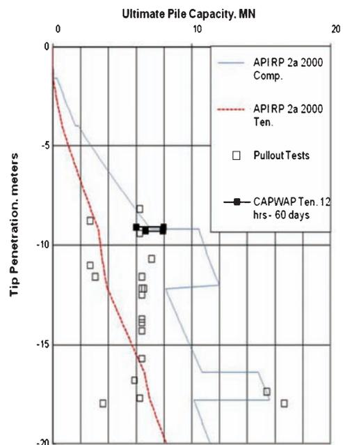
Figure 5. Pile capacity from API prediction, DMS results and pile pull out tests.
