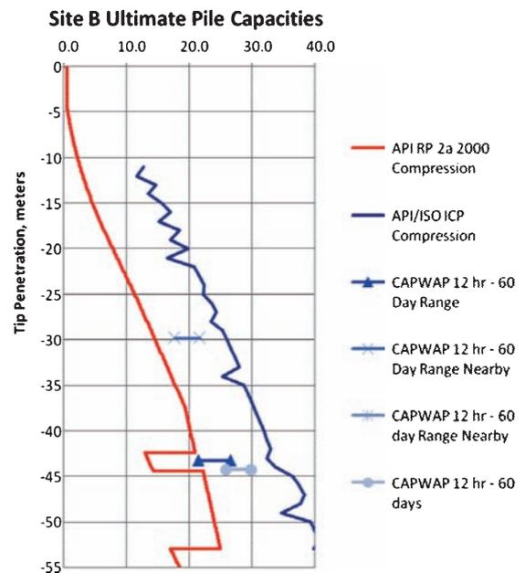
Figure 4. API, ICP and DMS pile capacities.
