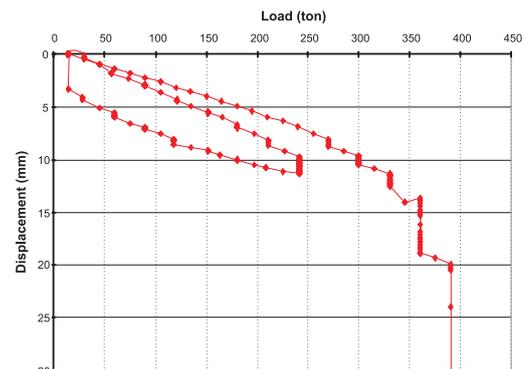
Figure 4. Static Load Test Case History 1.
