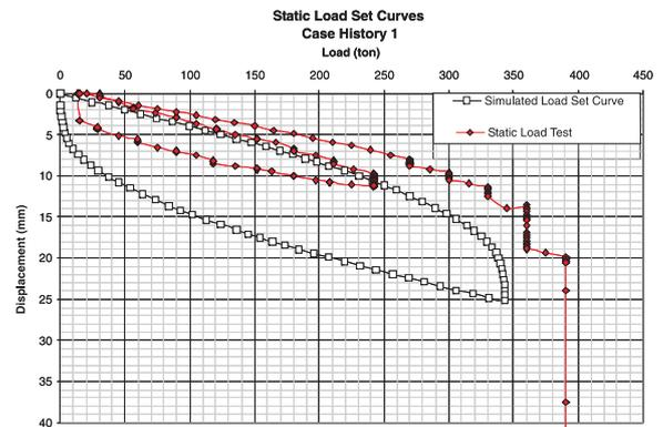
Figure 8. Static Load Test vs. Simulated Load Test.
