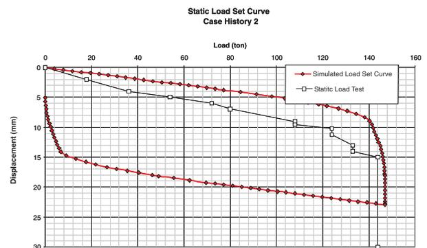
Figure 9. Static Load Test vs. Simulated Load Test.
