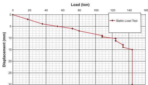
Figure 6. Static Load Test Results Case History 2.
