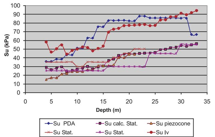
Figure 7. Shear strength  $S_u$  (kPa), obtained from static and dynamic tests, and computed considering the soil's viscosity index.
