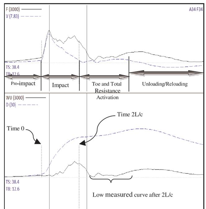
Figure 1. Force, velocity and wave-up records which show characteristically low measured response after  $2L/c$ .
