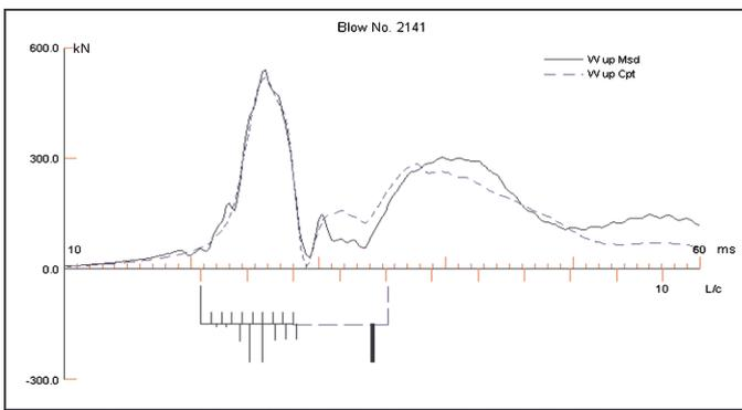
Figure 2(a). Final wave-up match plot using the standard Smith model (match quality of 3.94).
