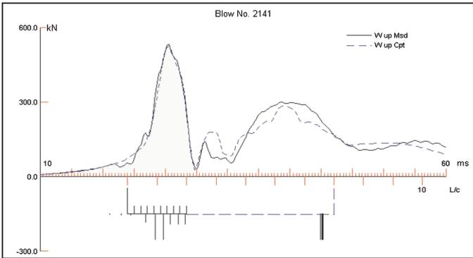
Figure 2(b). Final wave-up match plot using the radiation damping model (match quality of 2.89).
