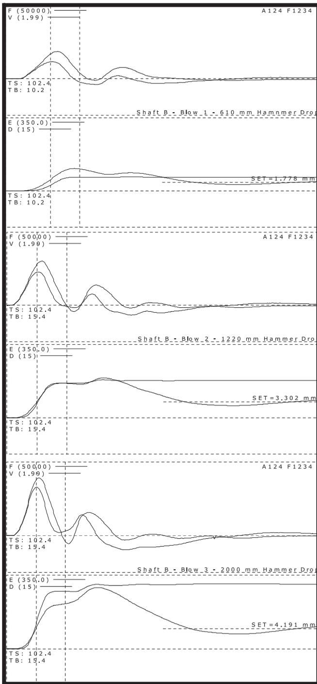
Figure 8. Plots of Shaft B test records for the three hammer test blows.
