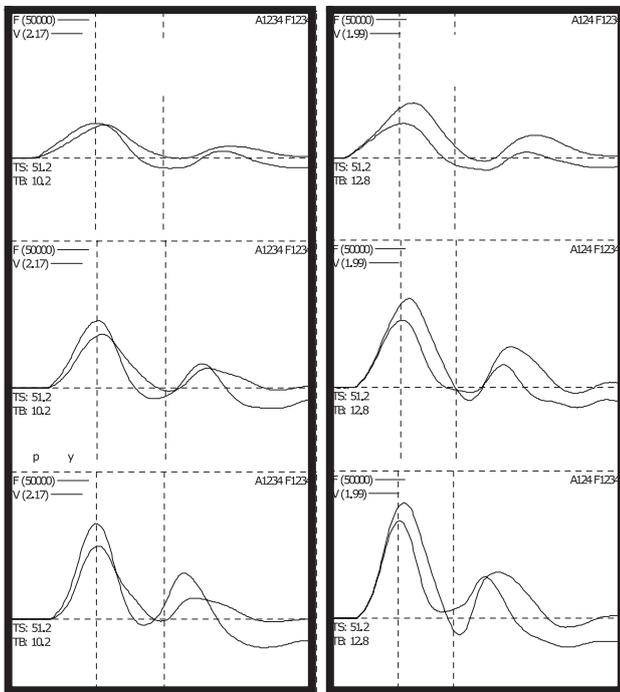
Figure 6. Plots of test records for Pier (left) and Shaft (right) B.
