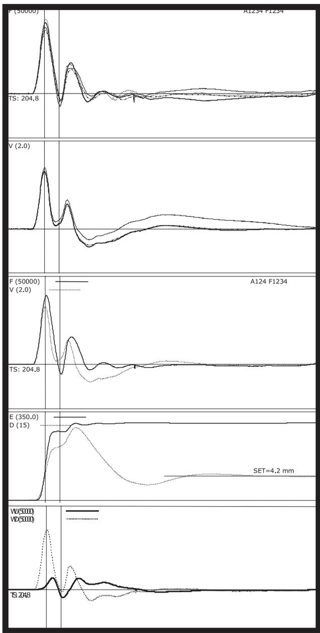
Figure 10. PDA data under blow 3 – Shaft B.
