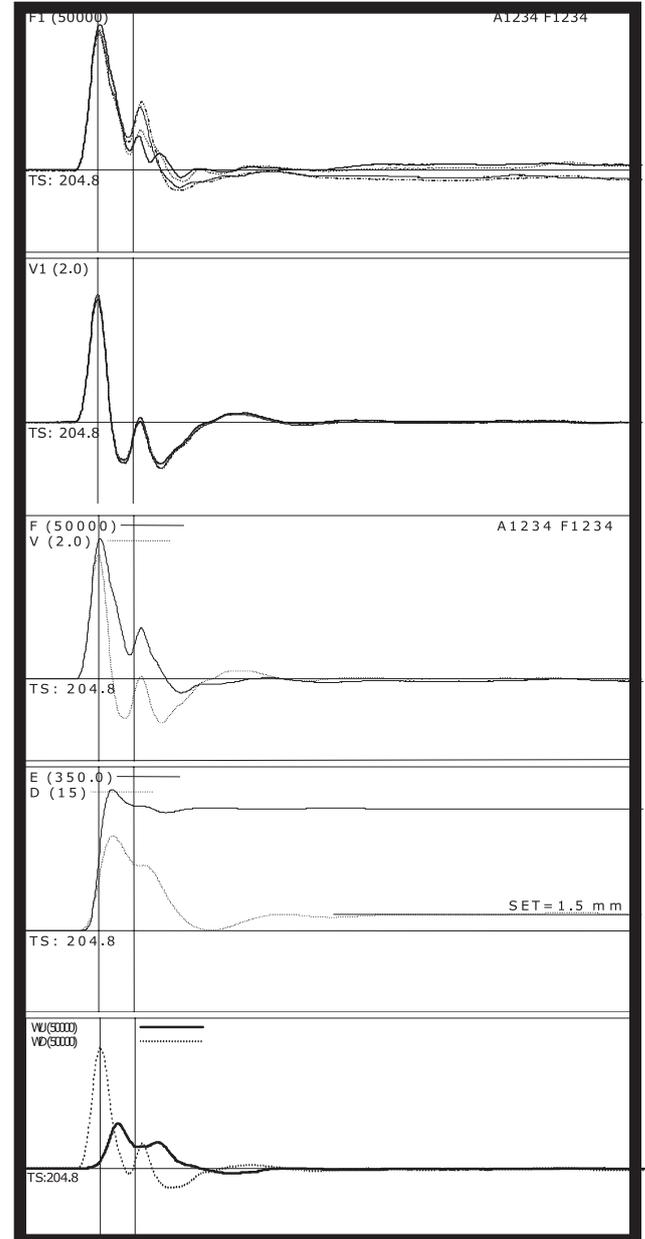
Figure 9. PDA data under blow 3 – Shaft A.
