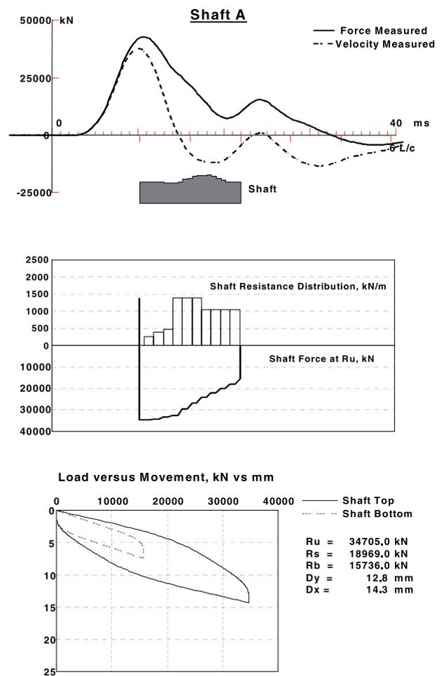
Figure 11. CAPWAP results – Shaft A.
