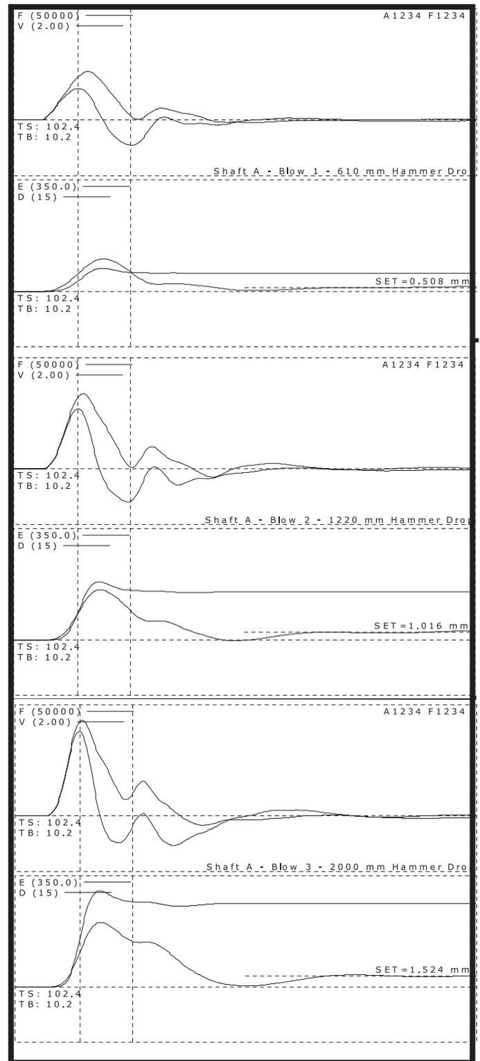
Figure 7. Plots of Shaft A test records for the three blows.
