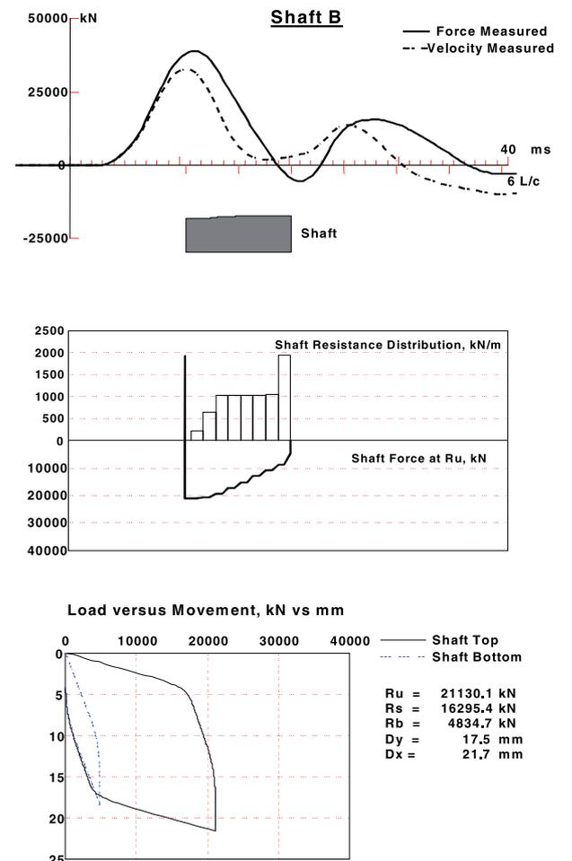
Figure 12. CAPWAP results – Shaft B.
