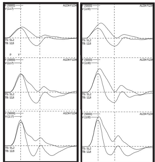
Figure 5. Plots of test records for Pier (left) and Shaft (right) A.
