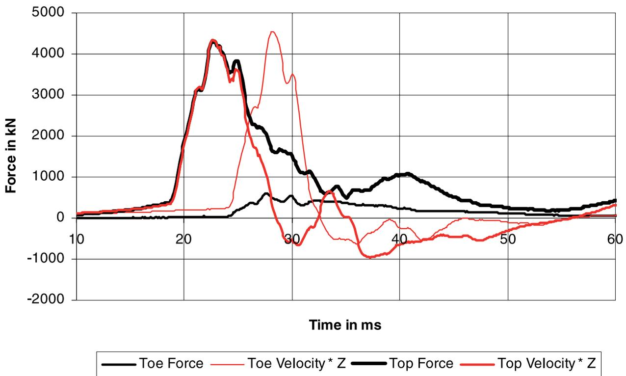
Figure 1. PDA top and toe measurements on a 450 mm square PSC pile.
