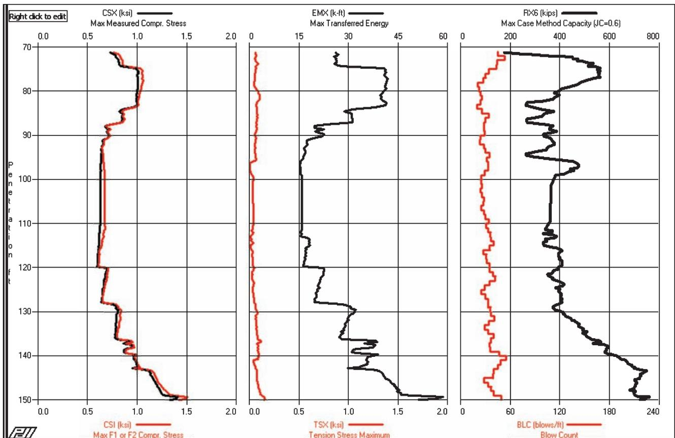
Figure 2. PDA graphical pile monitoring result summary.
