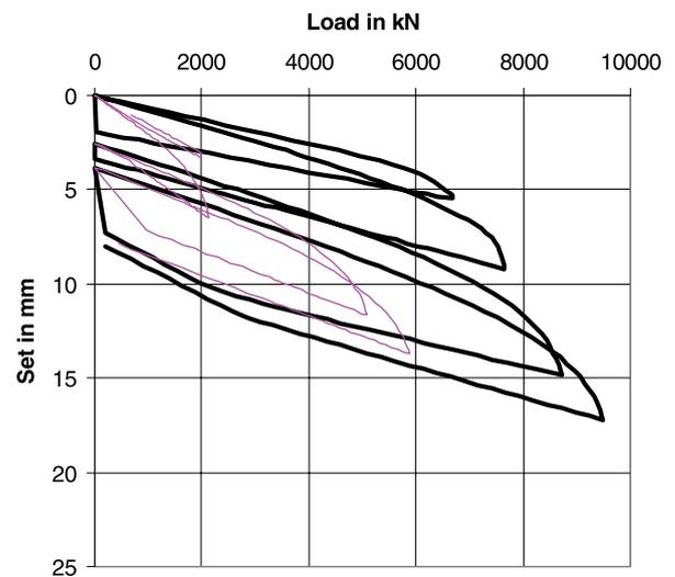
Figure 3. CAPWAP load-set curves for four consecutive impacts applied to a drilled shaft.
