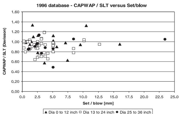
Figure 2. Ratio of CAPWAP to SLT prediction versus permanent set per blow.
