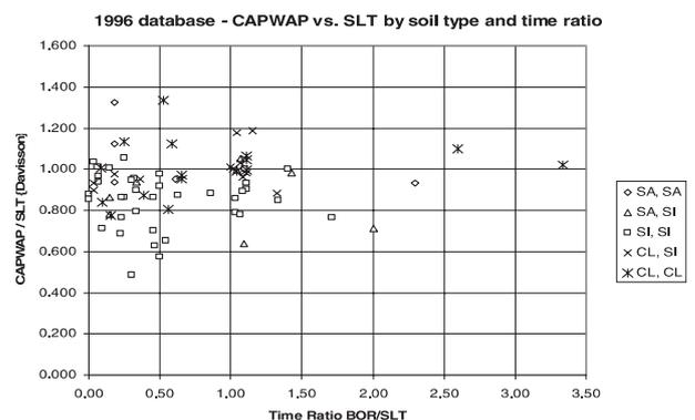
Figure 5. CAPWAP vs SLT by soil type and time ratio.
