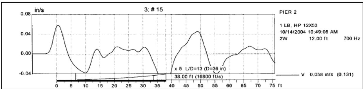
Figure 3. Pulse Echo Test on Steel Pile
