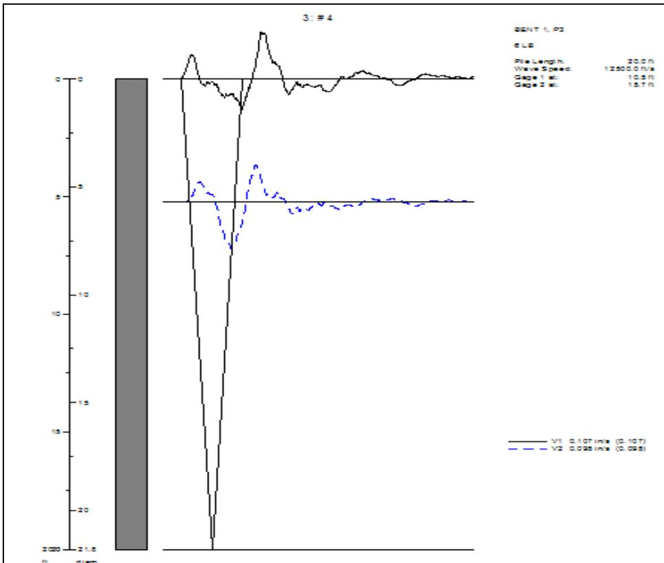
Figure 1. Two Velocity Signals in a Length-Time Plot from Pulse Echo Test on Concrete Pile
