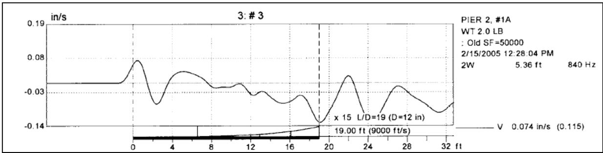
Figure 2. Pile Top Velocity from Pulse Echo Test on Timber Pile
