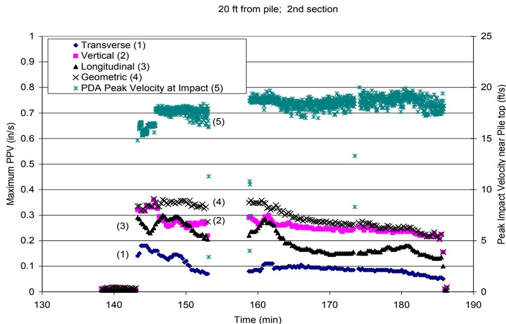
**Figure 4:** pile top and ground surface PPV values (Robinson 2006)
