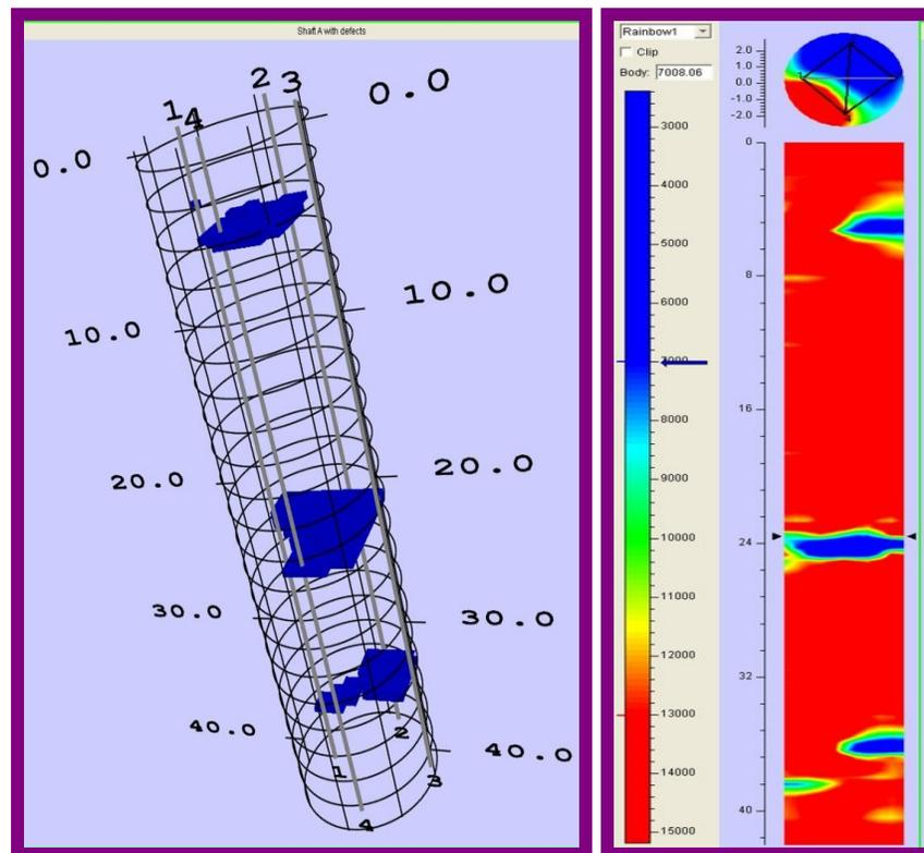
**Figure 9:** Tomography of a shaft with planned defects.
