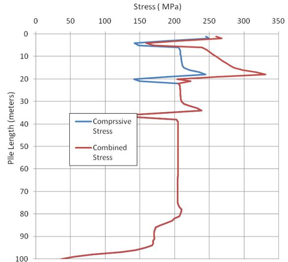
Figure 1 - Site A pile stress profile
