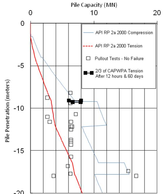
Figure 5 - Pile capacity from API, DMS and Pile pullout tests
