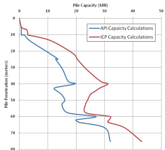
Figure 3 – API RP 2a and ICP pile capacity calculations
