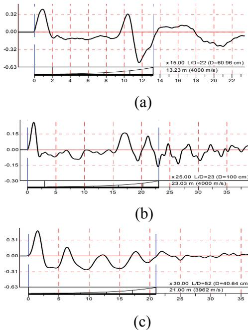
Figure 5. Examples of PD Category Records with significant positive reflections (SPR) assuming consistent magnification with other records at the same site: (a) No negative reflection before SPR at 9 m; (b) SPR near 15 m and only a small negative reflection (at 7 to 10 m); (c) SPR starting at 5 m followed by secondary reflections.
