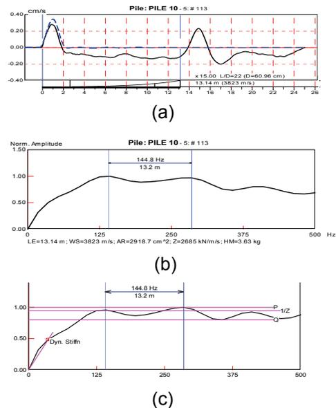
Figure 1. Example Record (ACIP; D=61 cm or 24 inch; L= 13.2 m or 43 ft): a) Time Domain Plot (Force dashed, velocity solid); b) Velocity Spectrum; c) Mobility
