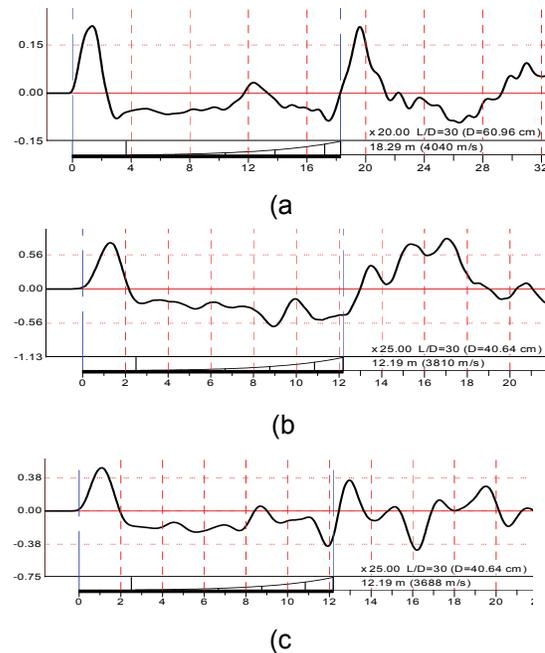
Figure 3. Examples of ACIP records (a)  $D=610$  mm (24 inch) and  $L=18.3$  m (60 ft); PF category, reduction beginning at 10 m; (b)  $D=406$  mm (16 inch) and  $L=12.2$  m (40 ft); AA category with bulge beginning at 8 m; (c) Pile as in (b) but PF category with impedance reduction beginning at 8 m.
