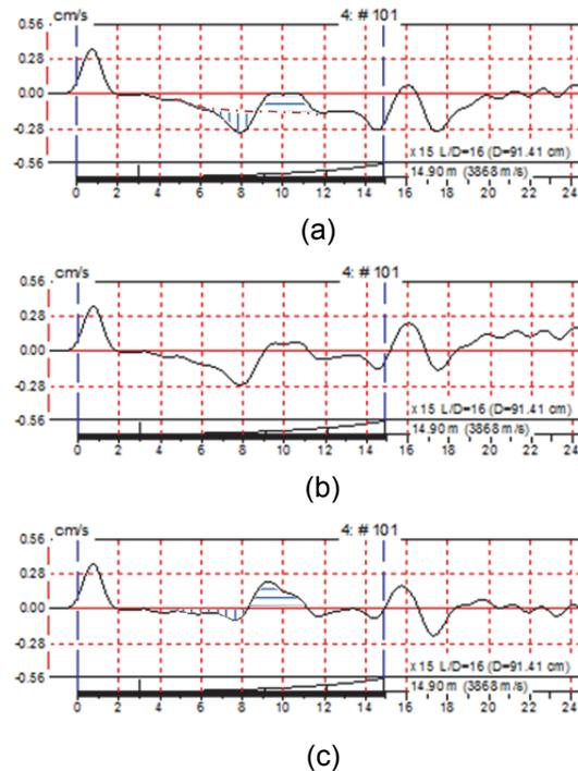
Figure 2. Example of Improper Use of High-Pass Filtering (ACIP Pile: Augured diameter = 750 mm or 30 inch): a) Without HI; b) HI = 200 m; c) HI = 15 m
