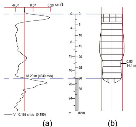
Figure 4. Profile Analysis for Record shown in Figure 3a: a) pile top velocity vs. time (downwards); b) estimated impedance profile indicating an estimated 17% reduction relative to pile top impedance.
