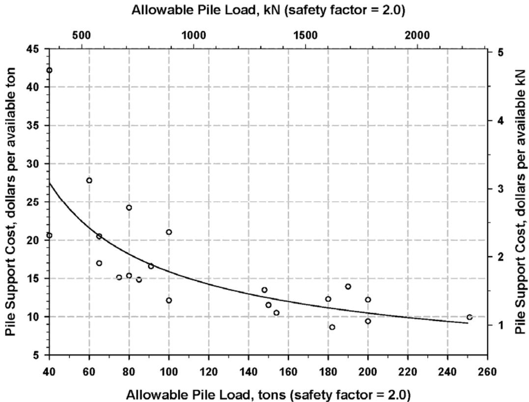
**FIG. 2. Pile Support Cost Based on Available Support vs. Allowable Pile Load (courtesy Wagner Komurka Geotechnical Group, Inc.)**
