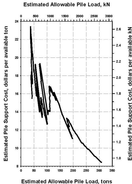
**FIG. 6. Pile Support Cost vs. Allowable Pile Load**
