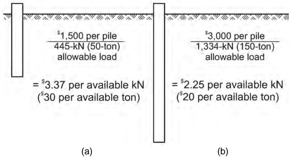
**FIG. 1. Examples of Pile Support Cost Based on Available Support**
