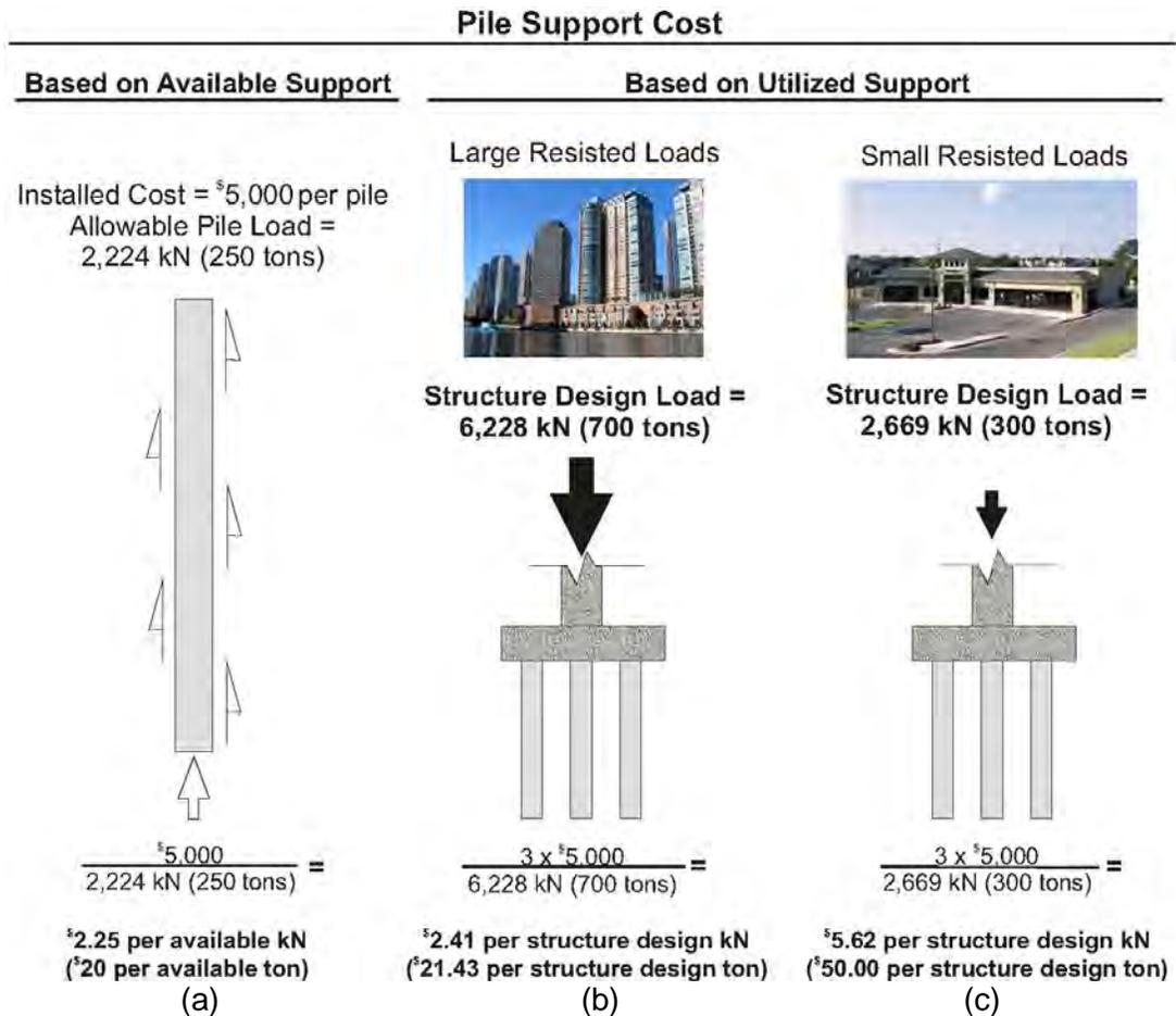
**FIG. 7. Comparison between Pile Support Cost Based on Available, and Utilized, Support**
