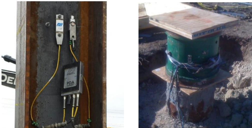
Figure 14: (a) Acceleration (right) and strain (left) transducers on pile to measure force and velocity, with wireless transmitter. (b) instrumented “top transducer”
