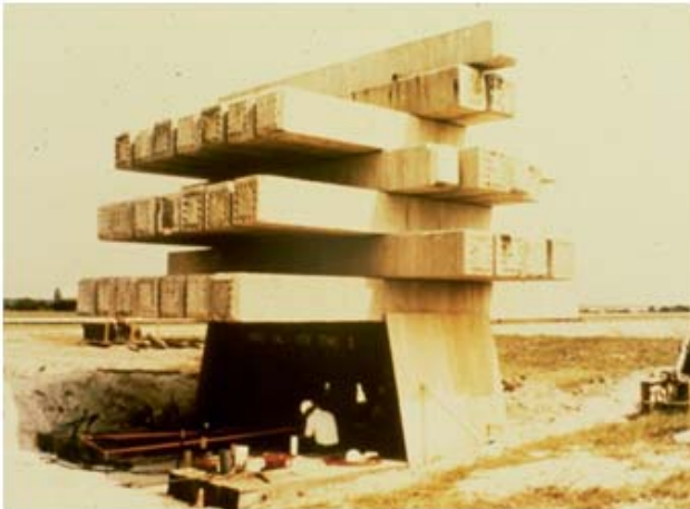
Figure 12: Static Load tests by dead weights (left) and reaction frame (right)
