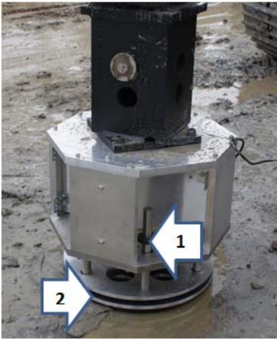
Figure 11: Shaft bottom quantitative inspection tool (cone probes measure force [arrow 1] while the bottom moveable plate measures deflection [arrow 2])
