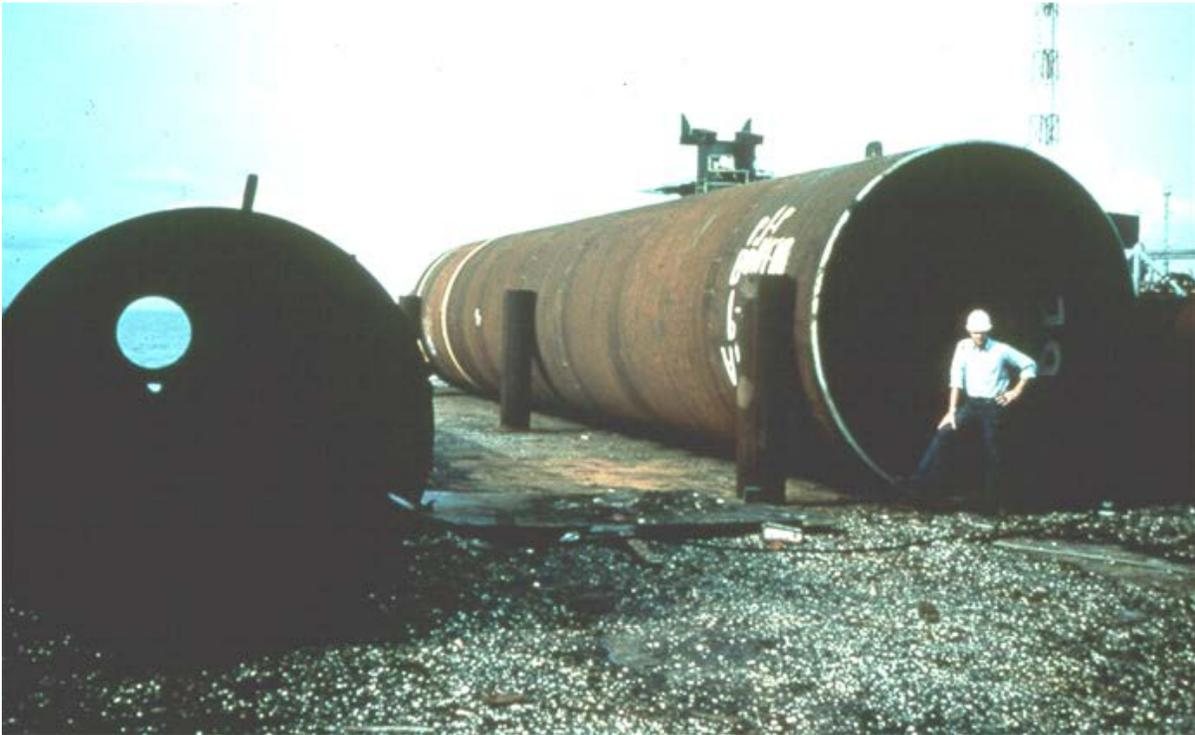
Figure 6-13 Large diameter open end pipe piles.
