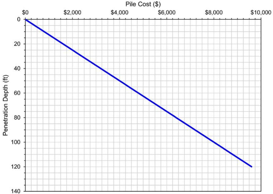
Figure 3-3 Pile cost versus pile penetration depth.
