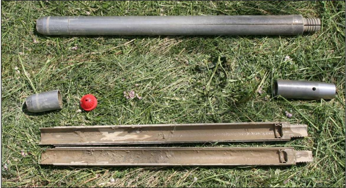
Figure 4-2 Standard split spoon sampler.
