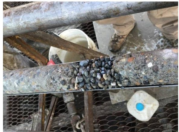
Figure 10. Core from Pier 9 Shaft C near EL.-87
