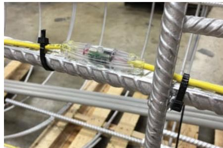
uate the positioning of the rebar cage and thickness of concrete cover. Concrete cover is of particular importance, structurally, in shafts subject to lateral loads such as those caused by wind. TIP using the Thermal Wire method consists of attaching specialty cables fitted with thermal sensors at every 300 mm along the
