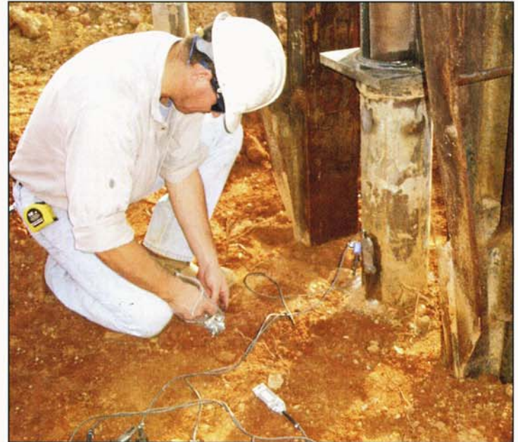
Scott Webster attaching a transducer on a micropile
