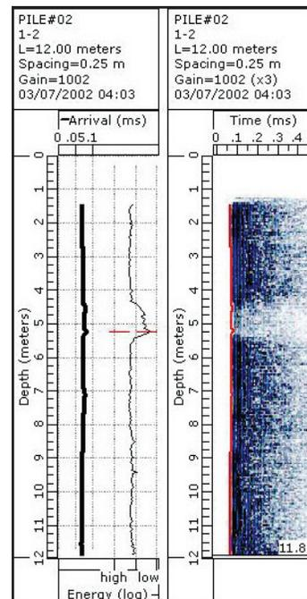
Figure 2: output of a CSL test between tubes 1 and 2 of the same 12m long defective at 5m shaft.
