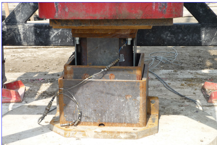
Figure 1: Load cell and cushion system on shaft top
