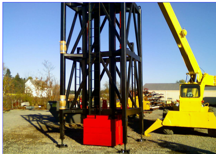
Figure 2: GRL's self-elevating 16-ton device
