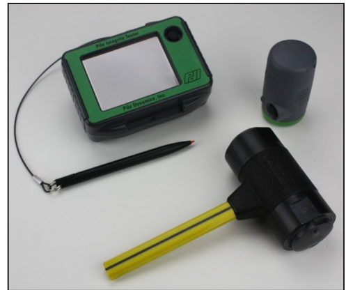
PIT-X with wireless accelerometer and handheld hammer.
