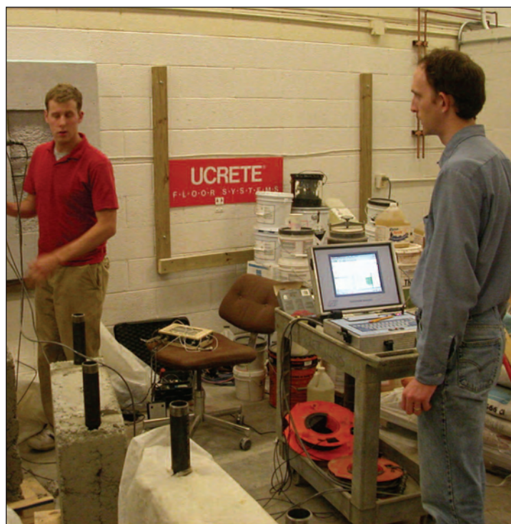
Eric Mack (left), Cleveland State University and Brent Robinson, formerly a GRL engineer who is currently at North Carolina State University, conducting CHA testing on a specimen of conventional concrete.
