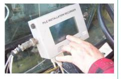
in the same manner and to the same standards as the test piles to insure production piles will also perform as well as the test pile. An automated monitoring equipment (like the PIR-A) documents that each production pile is installed with the same care and volume as the test pile.
