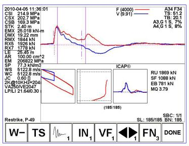
iCAP as seen on the screen of the PAX. Graphs, counterclockwise from top, are: Measured Signals; Simulated Static Load Test; Force in Pile Load Distribution and Signal Match
