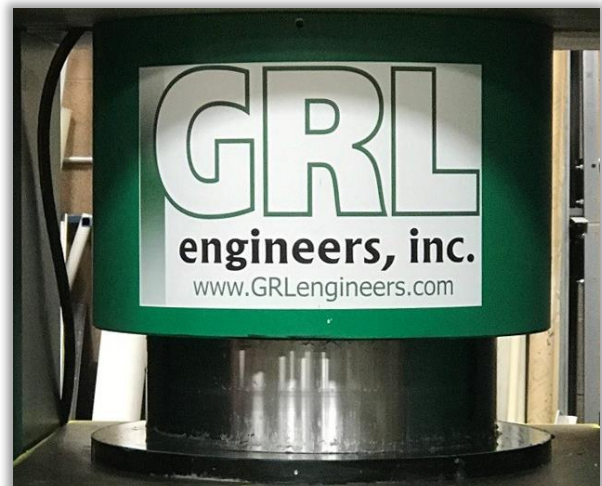
1100 Ton Cell Being Calibrated at 6 Inch Stroke
