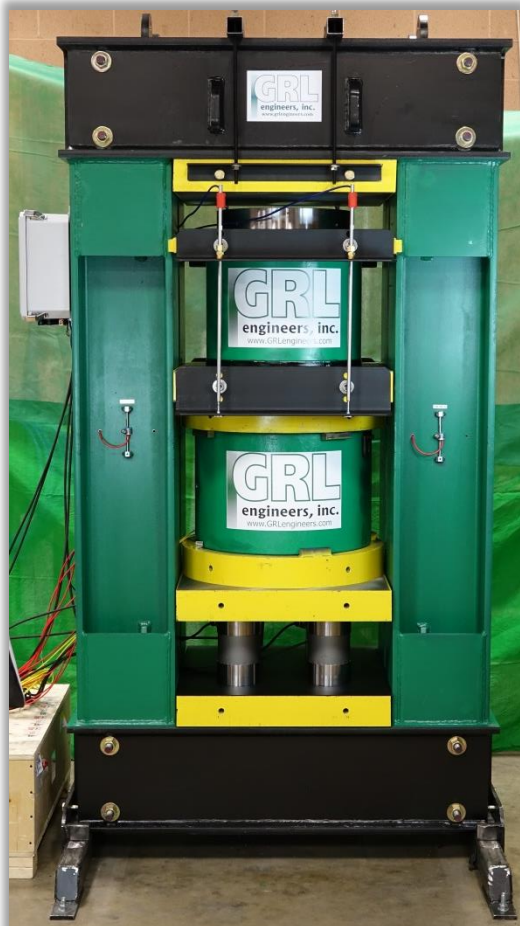
2000 Ton Load Frame with NIST Traceable Load Cells
