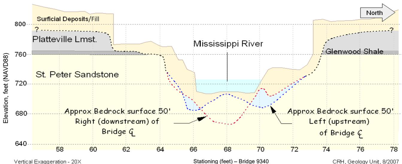
Figure 1. Generalized Subsurface Conditions (MnDOT, 2007)
