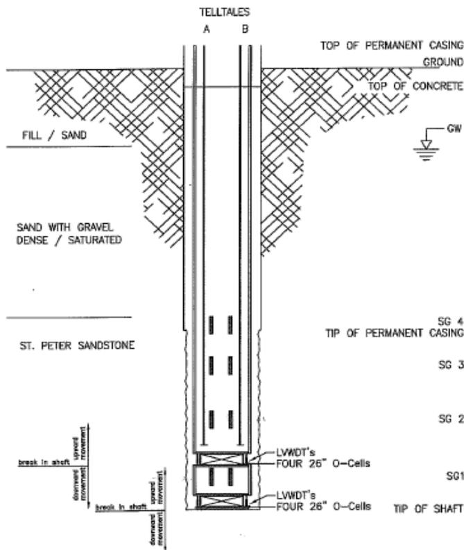
Figure 2. Test Shaft Arrangement (Loadtest, 2007)
