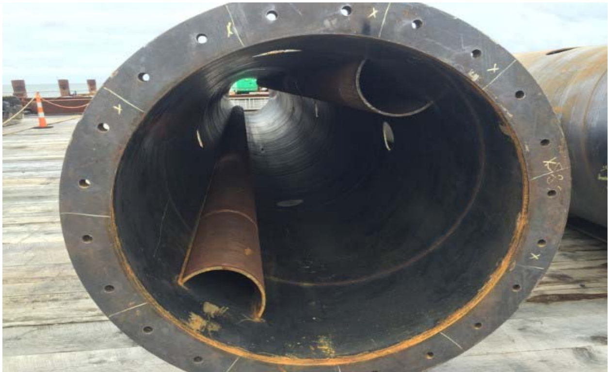
Figure 8. Steel pipe jetting and pile driving guide.
