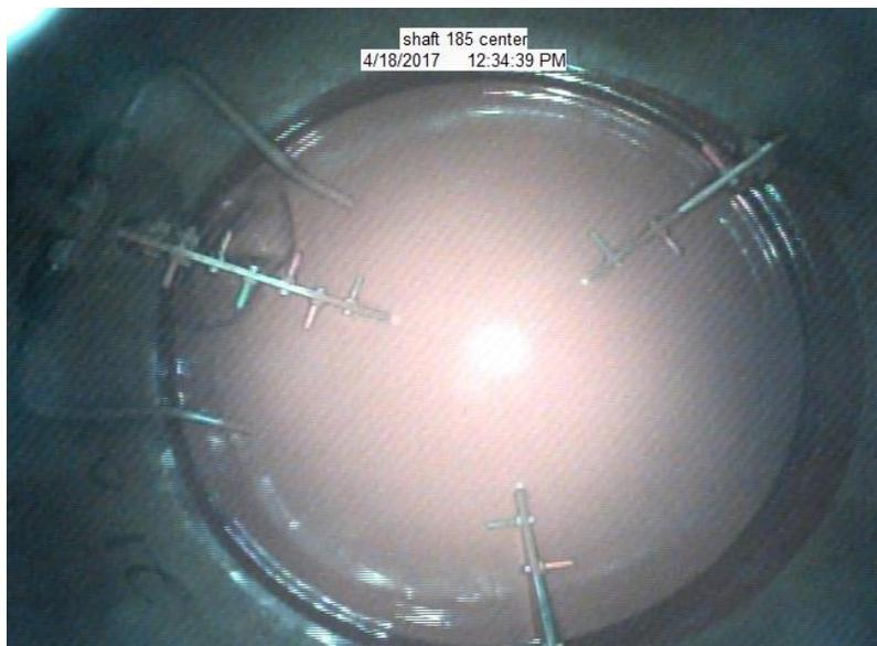
**Figure 2.** min-SID picture taken at the bottom of a drilled shaft, Ref. [4]
