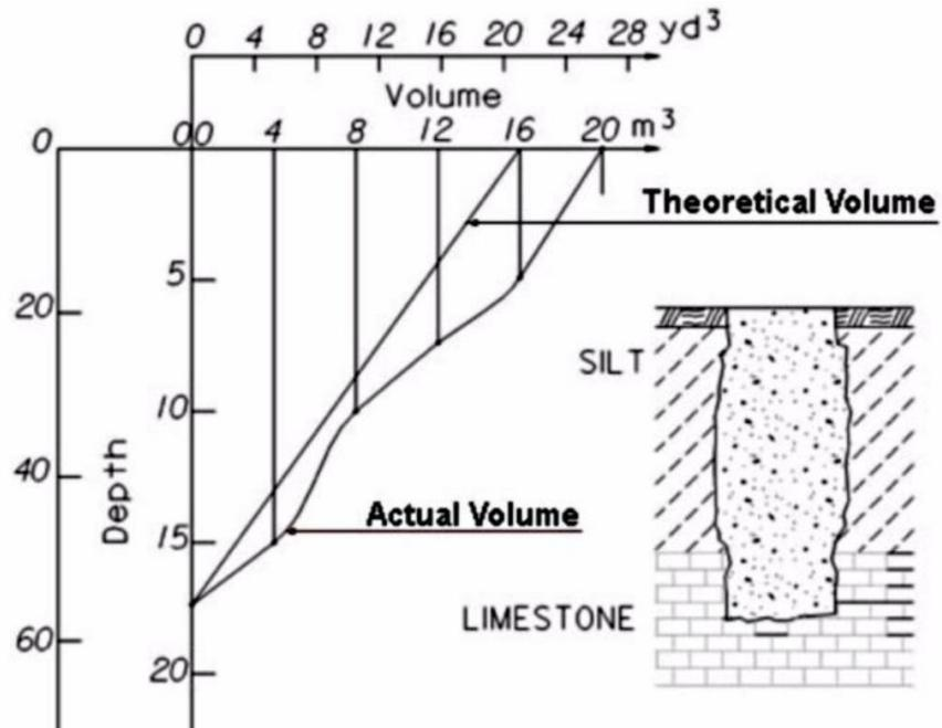
**Figure 9.** Concrete Volume-Depth Plot to assess drilled hole shape, Ref. [2]
