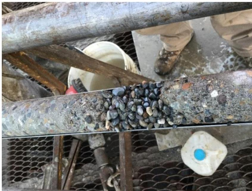
**Figure 8.** Coring results in a defective drilled shaft
