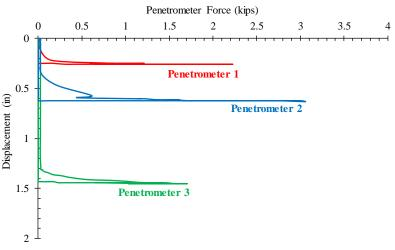
Figure 4. Penetrometer Force and Displacement plot from a SQUID Test
