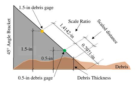
Figure 7. Mini-SID angle bracket details
