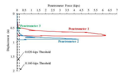
Figure 8. SQUID Test results for Drilled Shaft 161-Center
