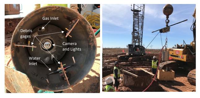
a) Camera and depth gages on a Mini-SID
