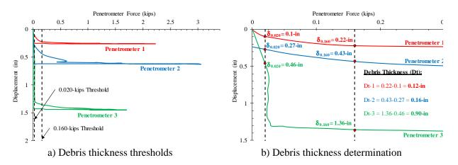
Figure 5. Force-Displacement plots obtained from SQUID testing
