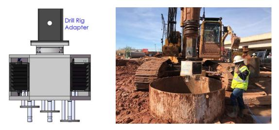
Figure 3. Shaft Quantitative Inspection Device
