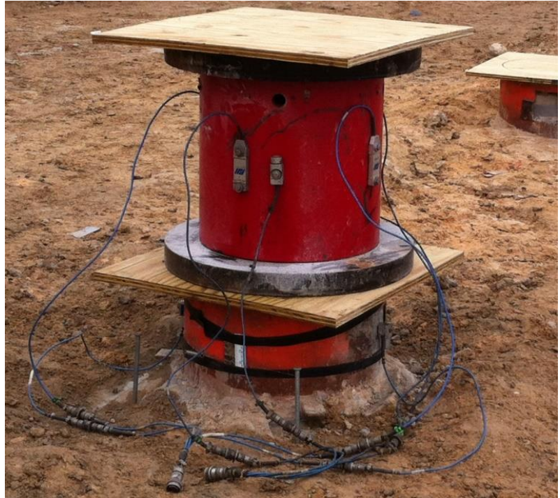
Figure 1 Transducer on top of a short pile top extension
