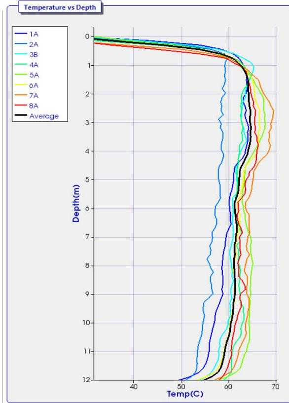
**Figure 3. Thermal results showing cage eccentricity**
