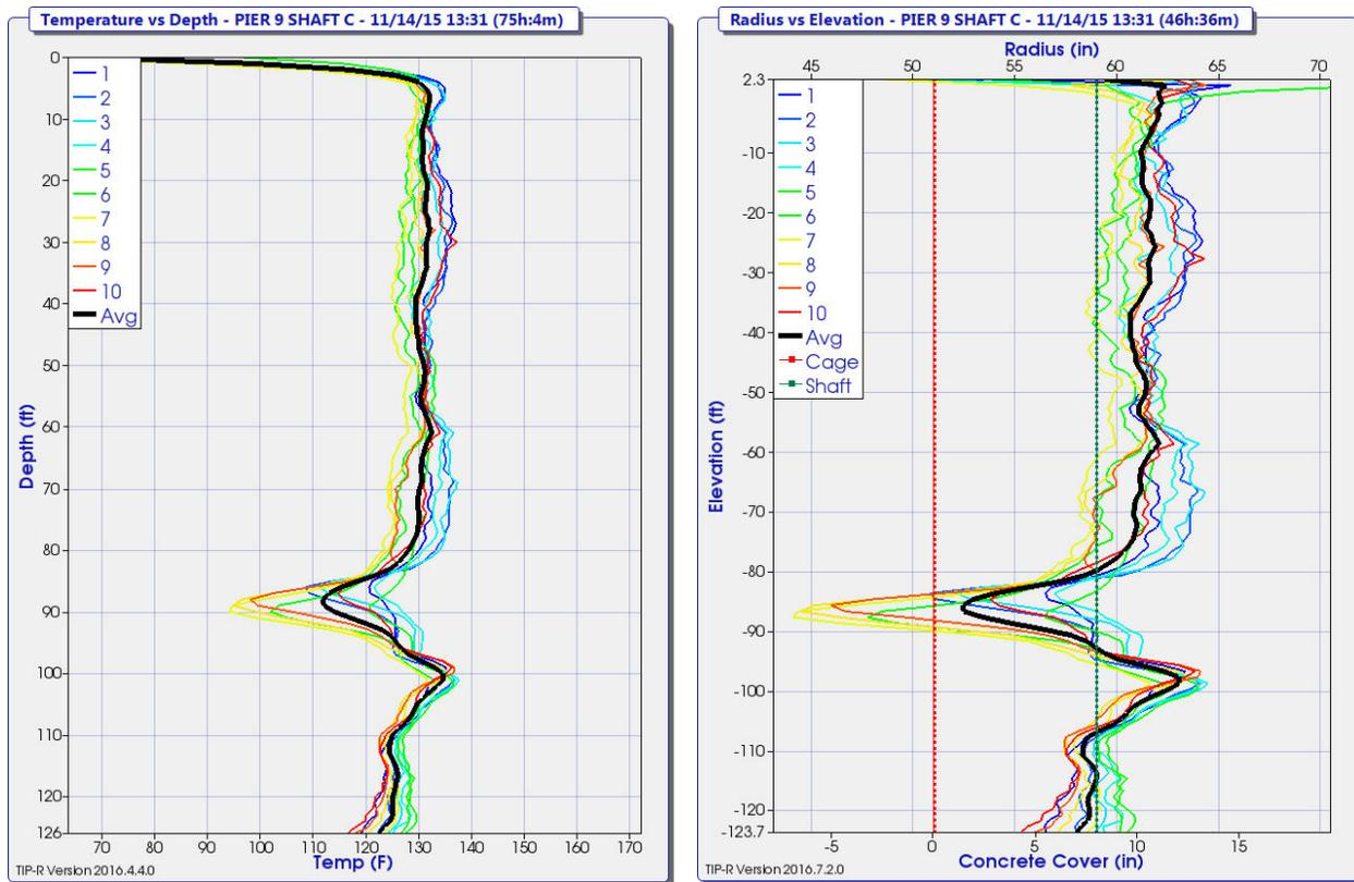
**Figure 2. Thermal results of temperature vs depth (left) and radius vs elevation (right) for the same drilled shaft with a defect at 27.4 m (90 ft.)**
