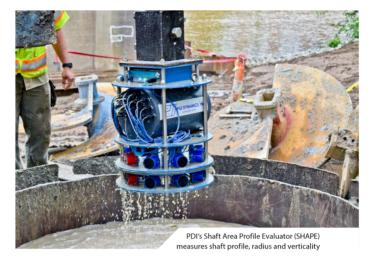
wireless capability allows the SHAPE data to be sent to the field tablet immediately upon exiting the excavation.
