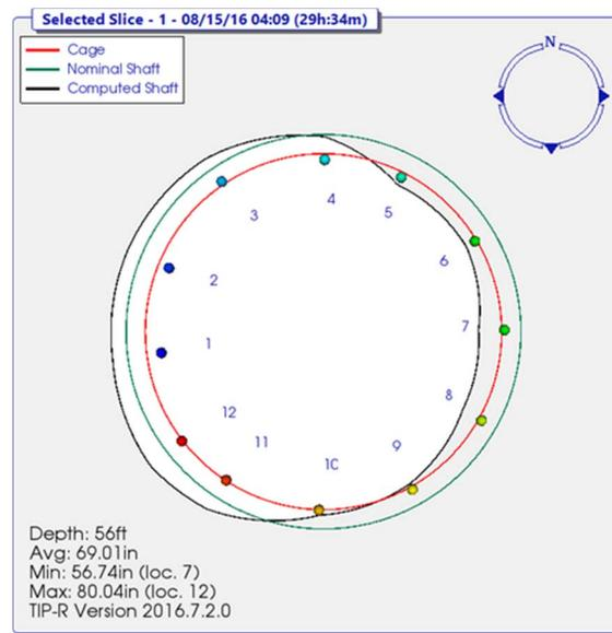
**Figure 10 – Cross-Section of Shaft 1 at 56-ft Depth (Bottom of Pier)**
