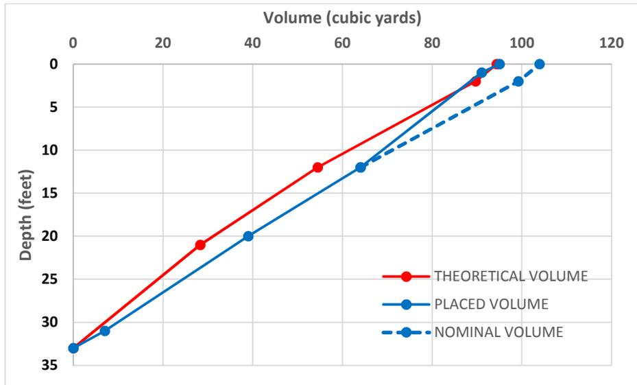
**Figure 5 – Shaft 2 Theoretical Versus Placed Concrete Volume**
