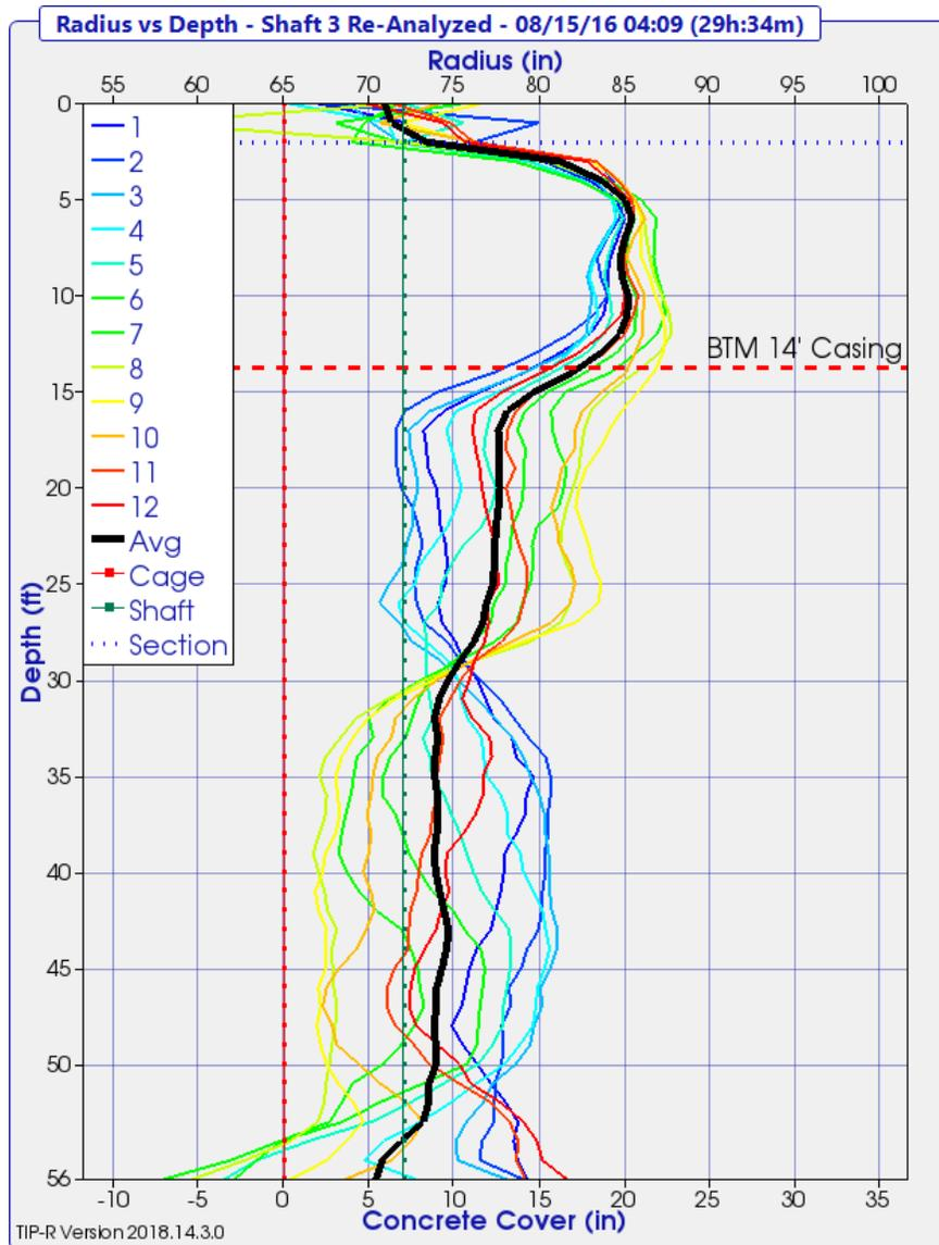
**Fig. 11– Shaft 3 Revised Effective Radius versus Depth**
