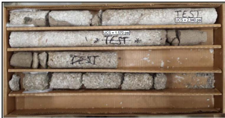
**Figure 6 - Shaft 2 Core Results**
