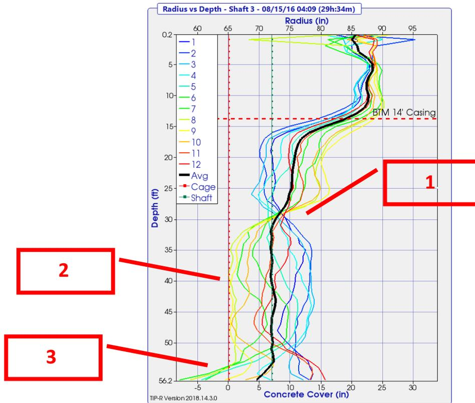
**Figure 8 – Shaft 3 Effective Radius versus Depth**
