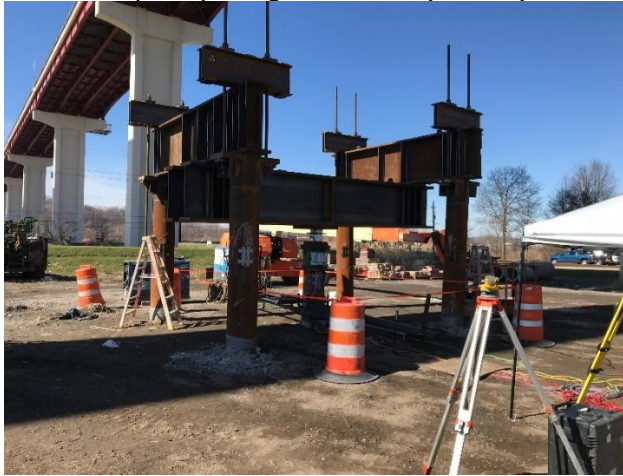
Figure 3: 2000-kip Static Load Test Frame (Top) – 56-kip Drop Weight Hammer (Bottom)
