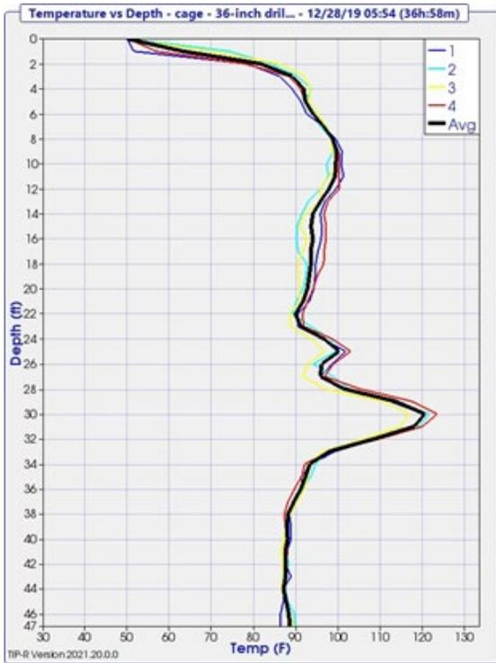
Figure 1: TIP Temperature vs Depth Rebar Cage Results
