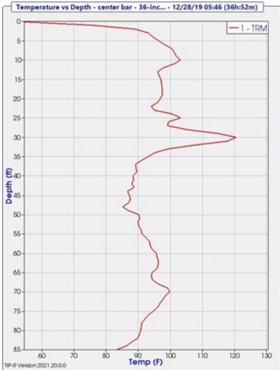
Figure 3: TIP Temperature vs Depth Center Bar Results
