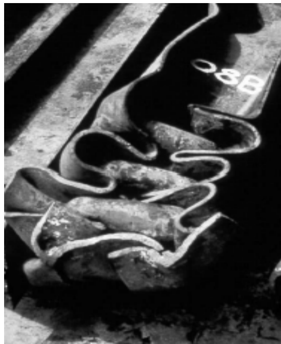
Figure 1. Damaged H pile.
