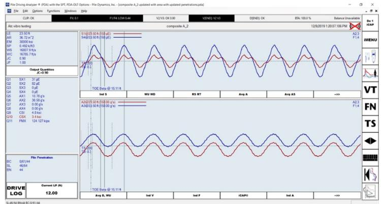
Axial stresses typically were less than 5 ksi during hard driving; during easy driving, stresses due to bending could reach almost 6 ksi. Maximum acceleration levels were less than 10 g's generally. Depending on soil resistance, hammer frequencies varied between 15 and 50 Hz.
