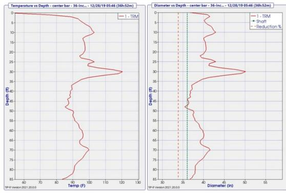
Figure 3: TIP Temperature vs Depth Center Bar Results
