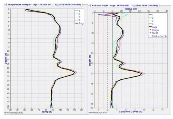
Figure 1: TIP Temperature vs Depth Rebar Cage Results
