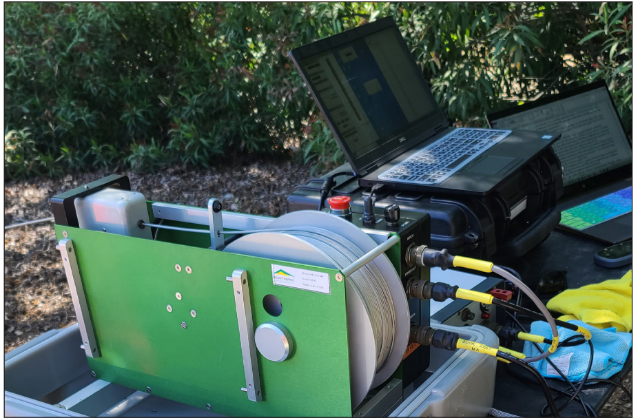
GGL system consisting of winch and data collection software
