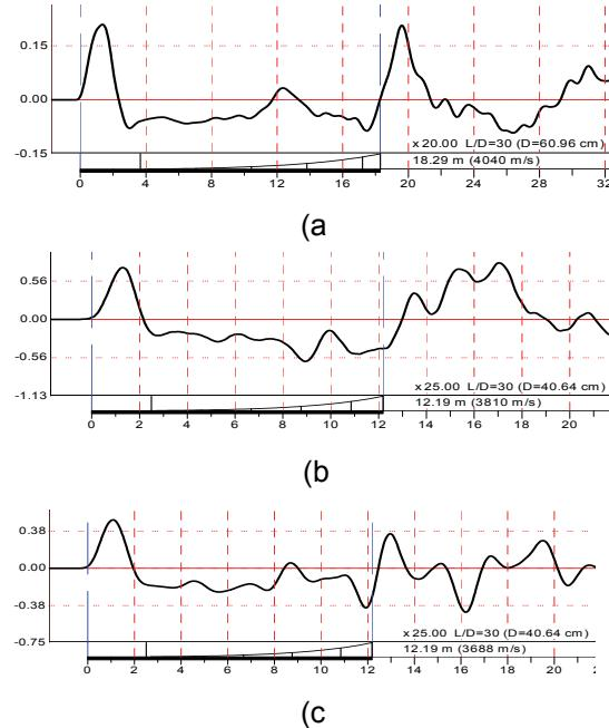
Figure 3. Examples of ACIP records (a)  $D=610 \text{ mm}$  (24 inch) and  $L=18.3 \text{ m}$  (60 ft); PF category, reduction beginning at 10 m; (b)  $D=406 \text{ mm}$  (16 inch) and  $L=12.2 \text{ m}$  (40 ft); AA category with bulge beginning at 8 m; (c) Pile as in (b) but PF category with impedance reduction beginning at 8 m.
