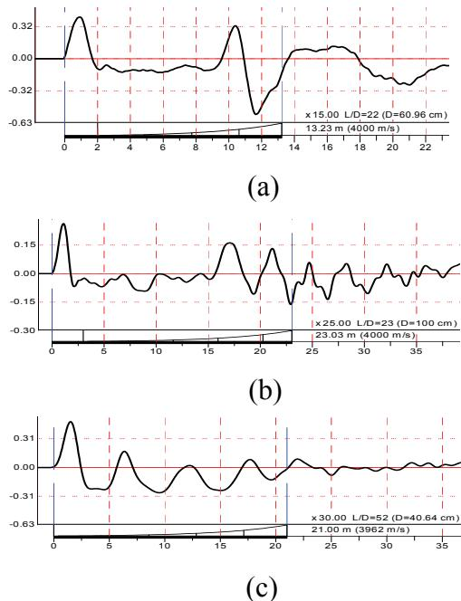
Figure 5. Examples of PD Category Records with significant positive reflections (SPR) assuming consistent magnification with other records at the same site: (a) No negative reflection before SPR at 9 m; (b) SPR near 15 m and only a small negative reflection (at 7 to 10 m); (c) SPR starting at 5 m followed by secondary reflections.
