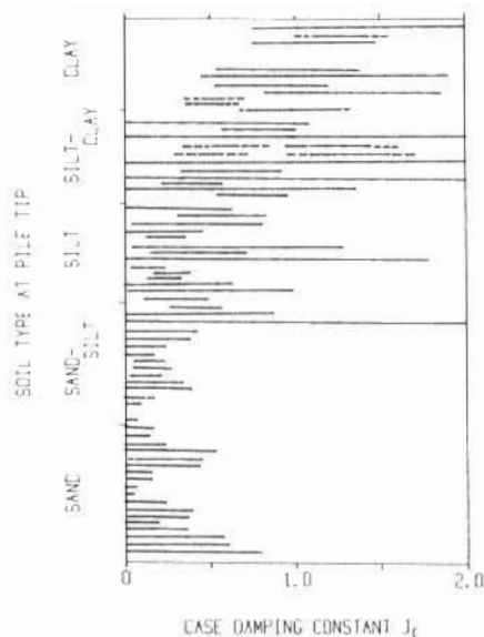
FIG. 7.—Damping Constant Determination by Correlation with Field Measurements
