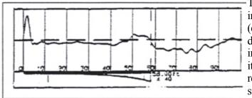
Figure 5: PIT Velocity versus Depth Record (Case 1)
