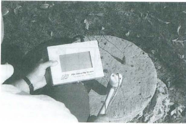
Figure 3. Pile integrity tester system.
