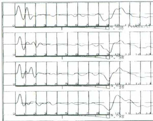
Figure 10: Accelerometer at center of 800 mm pile, hammer impact applied at N, S, W and E locations
