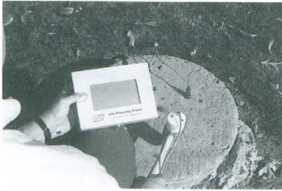
Figure 1. Pile Integrity Tester (PIT) with hammer and accelerometer for the application of the pulse echo method.
